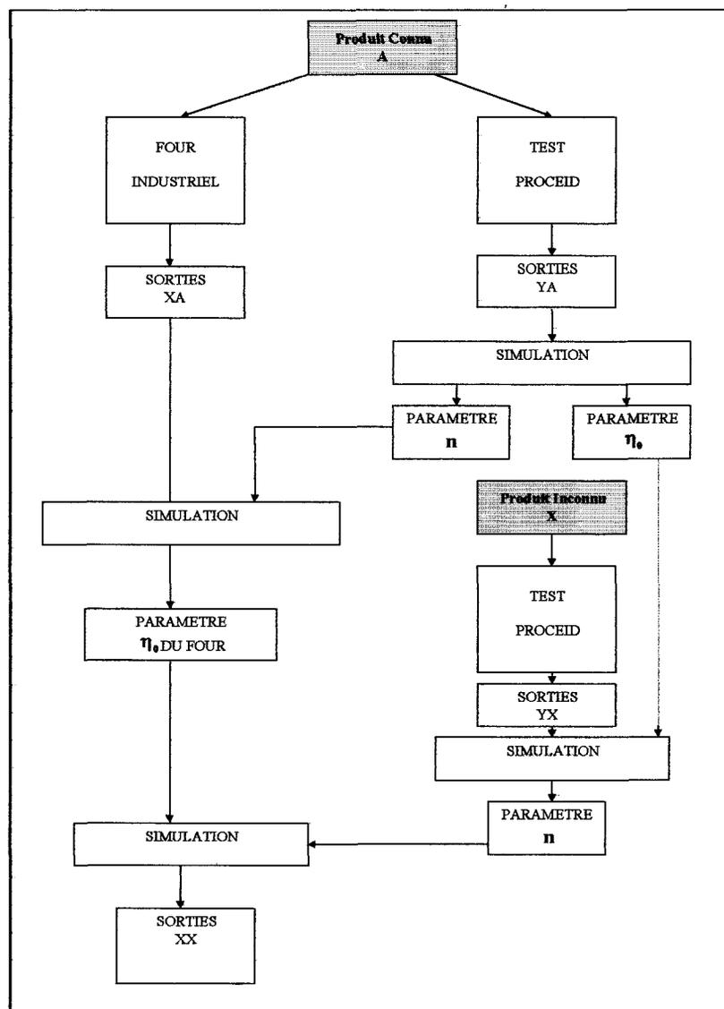
This extrapolation procedure permits the performances prediction for waste thermal destruction together with the corresponding emission evaluation on a large scale facility, starting from pre-test conducted on the PROCEED bench. The precision obtained is around 10%.
