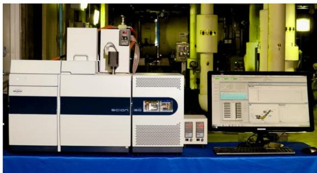
Figure 61 : On-line trace siloxane analyzer (Lotus Instruments).
