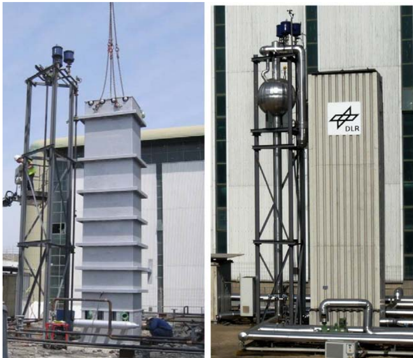
Figure 52 : PCM test module at the test site (with and without insulated) [8]
